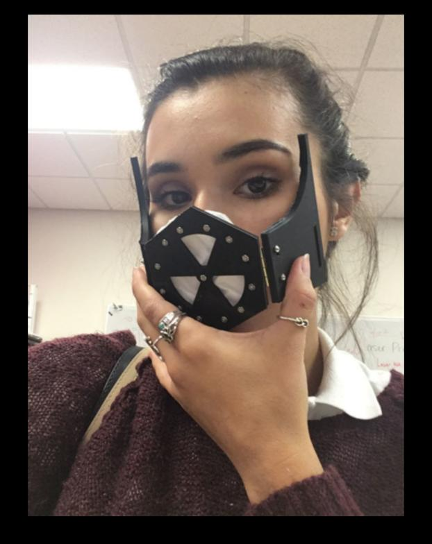
Fourth Iteration: 3D printed, made out of plastic. Added real filter that filters sand and germs. Screwed the filter onto the printed parts.
